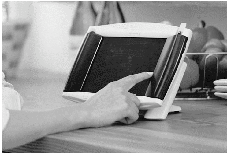
Figure 2: Ericsson Cordless Screen Phone HS210 with Internet Access, e-mail, and telephony using Bluetooth wireless communication (from http://www.ericsson.com/cebit/webcast/sld005.htm )
