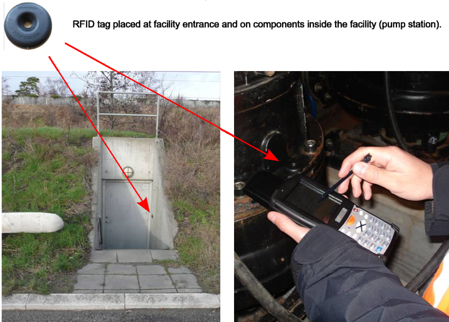
Figure 1 Illustration of rugged RFID tags placed at the entrance to the facility and the PDA with RFID reader used for the implementation of SMART Mobile RFID.
