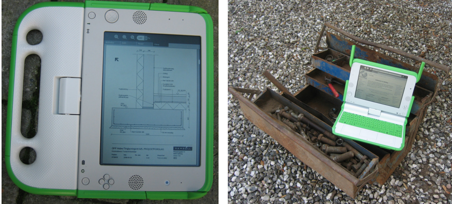
Figure 16 Illustration of how the OLPC can be used for displaying construction details and work instructions.
