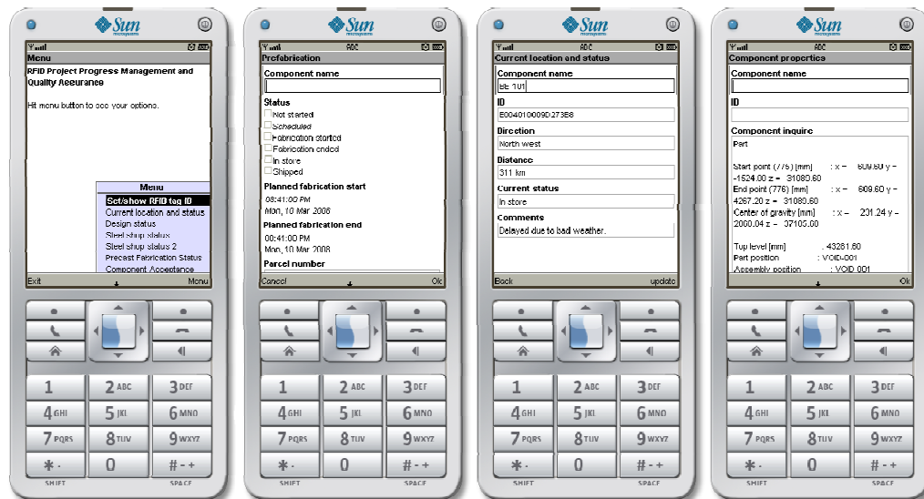
Figure 7 Screen dumps from a mobile phone based prototype application for project progress management and quality assurance. The screen dumps are from mobile phone emulator executed on a PC. From left the screen dumps show 1) a part of the menu, 2) input window used by the manufacturer of prefabricated components, 3) output from an inquiry of a component's current location and production status, and 4) output from a full component attributes inquiry.
