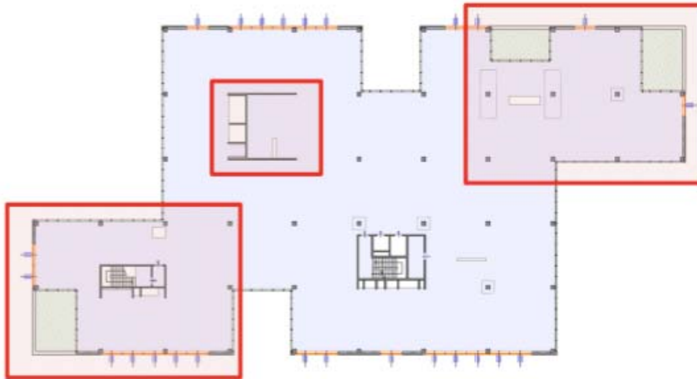
Figure 398 – By combining several “Boundary Filters” by setting the “Consider” option to “Any”, you can specify multiple areas in your project under one Location in your WBS. A “Zone C” could, thereby, consist of three Zones in a floor plan.
