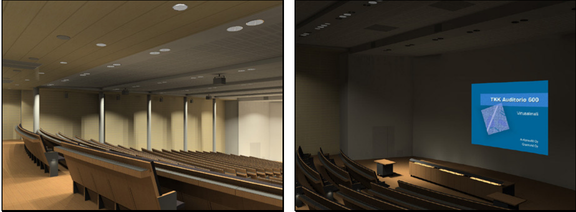
Figure 13. LIGHTSCAPE renderings showed the end-users the proposed lighting designs for the auditorium hall in lecture mode (left) and slide presentation mode (right).
